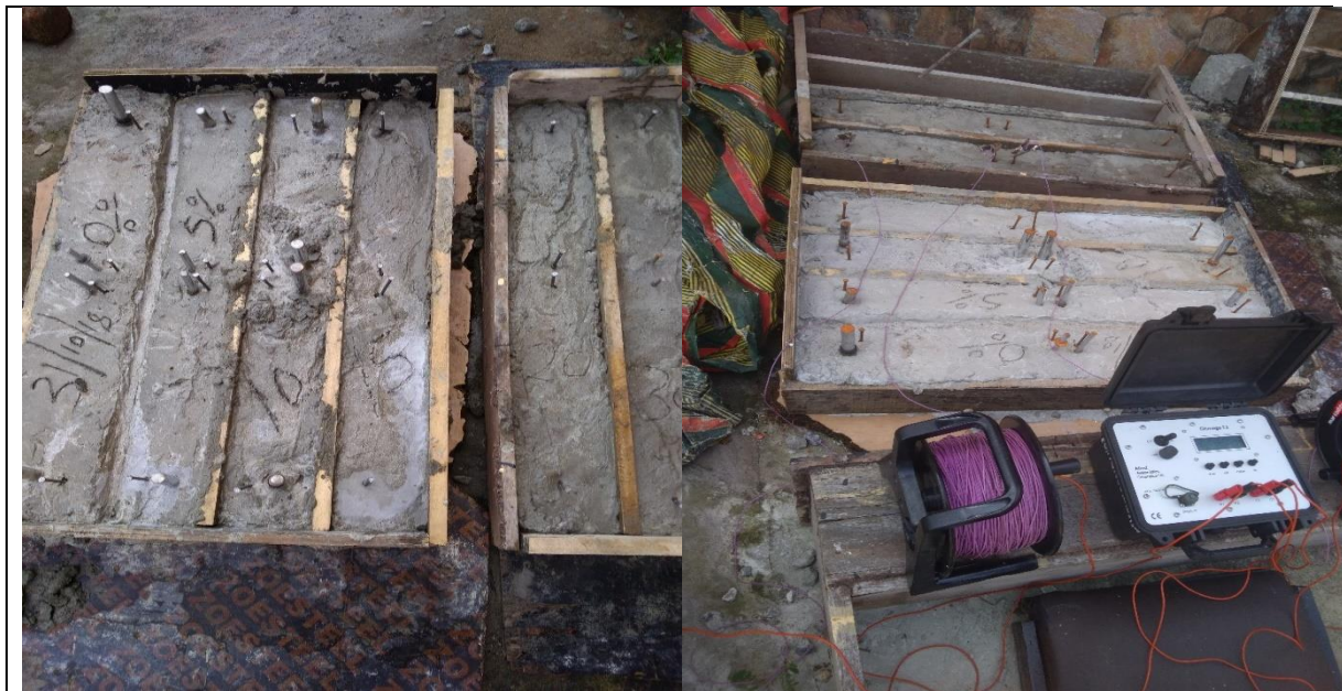
Figure 2: Concrete cast with electrodes inserted for electrical resistivity test
