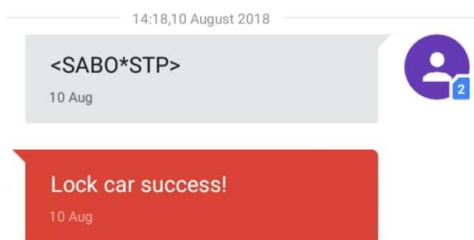
Figure 9: Message from the Speed Limiter after Sending the STOP Code
