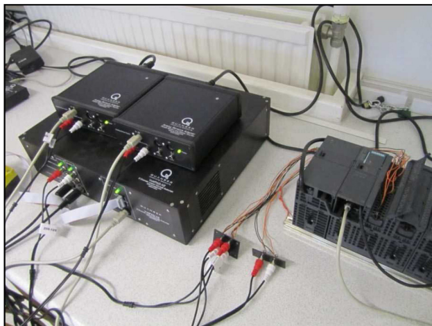
Fig. 4. Wiring between the Siemens PLC and the Quanser board (from Date, 2012).
