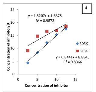
Figure 4 represents Langmuir isotherm for Corrosion of Zn alloy in the presence of lantana camara in 2M H<sub>3</sub>PO<sub>4</sub>
