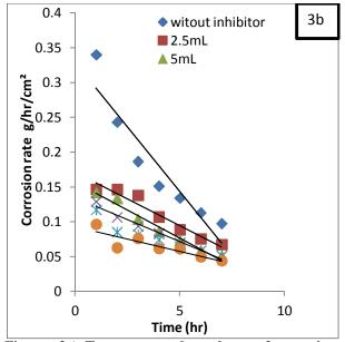
Figure: 3a) Temperature dependence of corrosion rate of Zn alloy and 3b) is Corrosion rate of Zn alloy at 303K in 2M H<sub>3</sub>PO<sub>4</sub>
