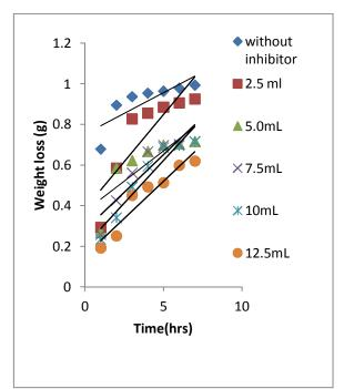
Figure 1: Variation of weight loss of Zn alloy with time in the presence and absence of lantana camara at 303K in 2M H<sub>3</sub>PO<sub>4</sub>
