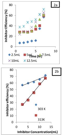
Figure 2a: Variation of inhibition efficiency of lantana camara with time at 303K. Figure 2b: Temperature dependence of inhibitor efficiency of lantana camara in 2M H<sub>3</sub>PO<sub>4</sub>
