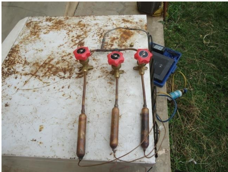
Figure. 4: Experimental Setup of Different Capillary Tube Length of 1.5m, 2m and 3m
