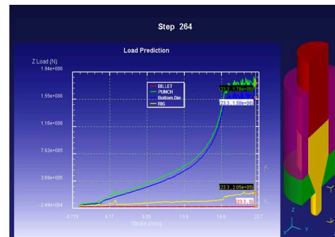
Fig. 18 Variation of punch load with respect to punch travel for extrusion of circular section
