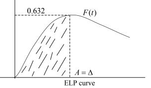
i.e.63.2% life span of the equipment has expired .At this state the equipment is fatigued and most likely prone to corrosion.
