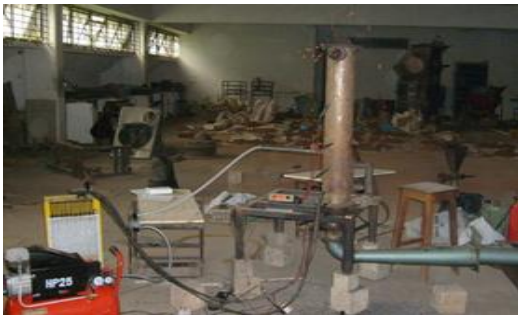
Plate 1: Fabricated fluidized bed combustor setup
