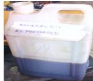
(e) Mineral Oil Cutting Fluid (MCF)
