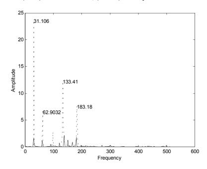
Figure 6: Comparison of vibration spectra due to mechanical looseness; (solid) - FFT estimates, (dotted) - ARMA spectra estimates (solid) - FFT estimates, (dotted) - AR spectral estimates
