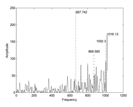
Figure 4: Comparison of vibration spectra due to gear fault; (solid) - FFT estimates, (dotted) - AR spectral estimates
