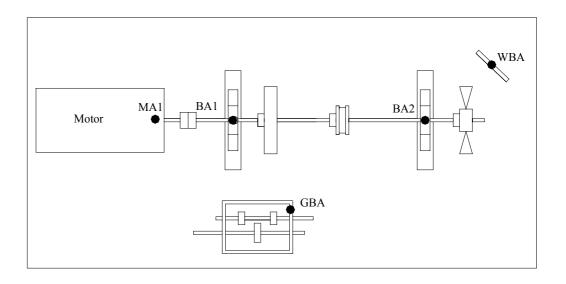
Figure 1 : Accelerometer mounting positions
