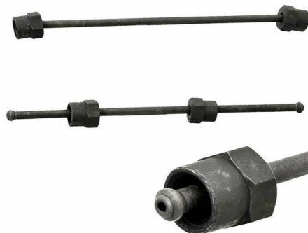
Figure 2.4: Metallic fuel lines.
