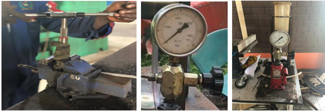
(d) Threading the piston (e) Pressure gauges after coupling (f) Mounting on the base
