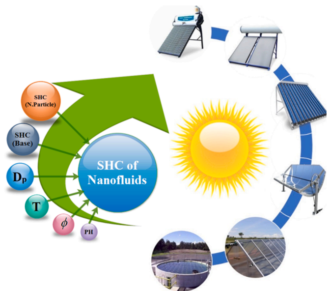
Fig. 1. The schematic view of nanofluids application in the solar energy systems and influence factor in Specific heat capacity of nanofluids.
