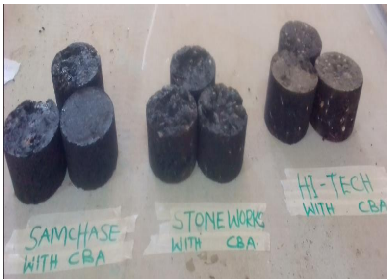
Fig. 3. Asphaltic concrete samples with CBA.
