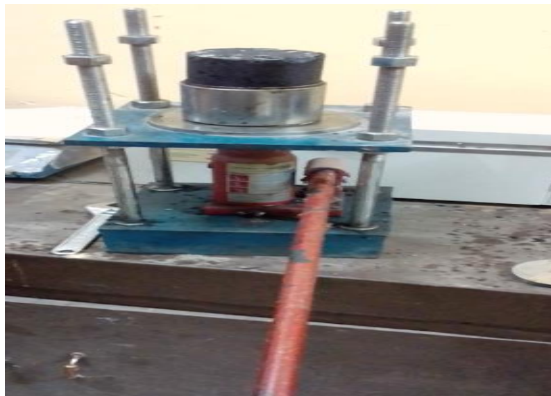
Fig. 3. Extruding the asphaltic concrete.
