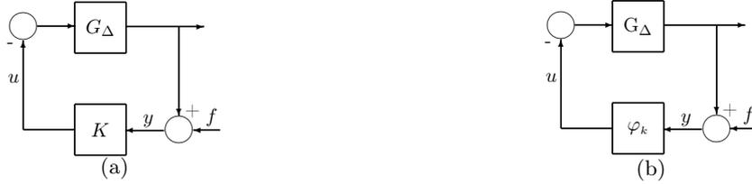
If the system in Fig. 4.7(a) is stable, then system in Fig. 4.7(b) is stable.
