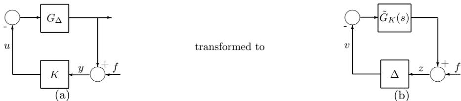
Using LFT, the system in Fig. 4.4(a) is transformed into Fig. 4.4(b).
