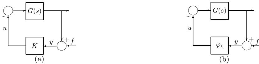
If the system in Fig. 4.2(a) is stable, then system in Fig. 4.2(b) is stable.
