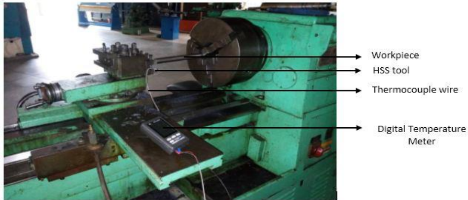
Figure 3: Experimental set up for machining process
