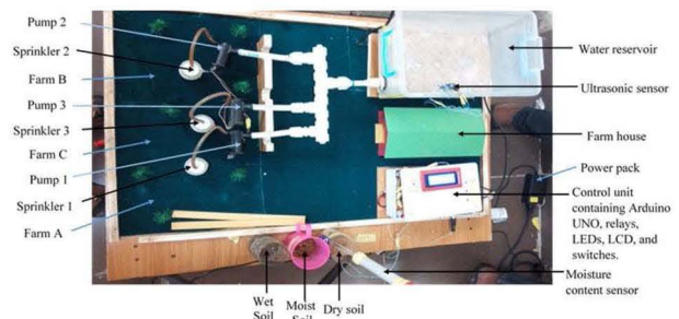
Fig. 5: Developed laboratory-scale smart irrigation system
