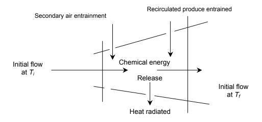
Fig.3 : Heat balance for a thin flame
