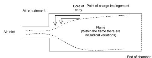
Fig. 2: Combustion Chamber with assumed flow pattern.
