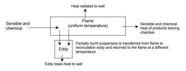
Fig. 4: Combustor sample for isothermal version
