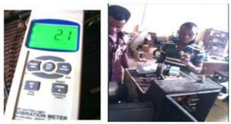
Fig. -5: Portable Digital SD Card Data Logger Vibration Meter (VB 8206SD)
