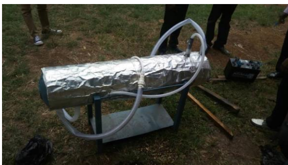
Fig. 9: Field Test Demonstration of the STHE
