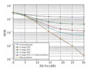
Figure 4. BER versus Eb/No with perfect channel estimation under Flat fading MIMO channels.
