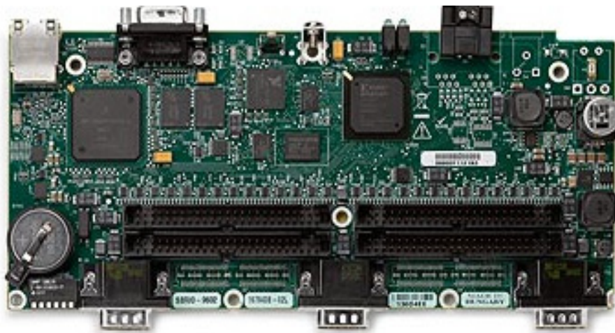
Figure 4. NI sbRIO-9642 for real-time hardware target
