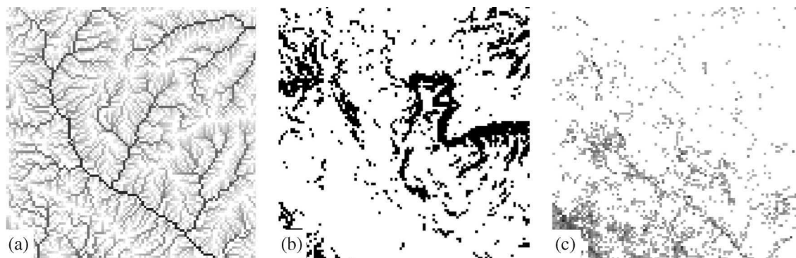
Fig. 5. Maps of (a) upstream area, (b) slope, and (c) NDVI for the Ejura study-site window (10 × 10 km). For the slope, a threshold of 2% has been applied, and for NDVI, a threshold of 0.049 has been applied.
